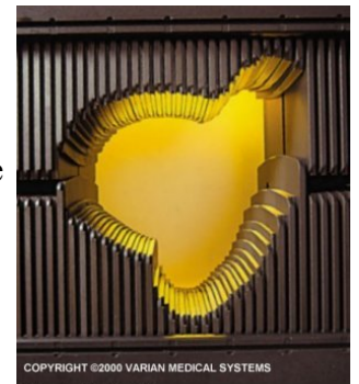
An image of the Varian Multileaf Collimator which shapes the radiation beam in accordance with the most optimized treatment plan.
